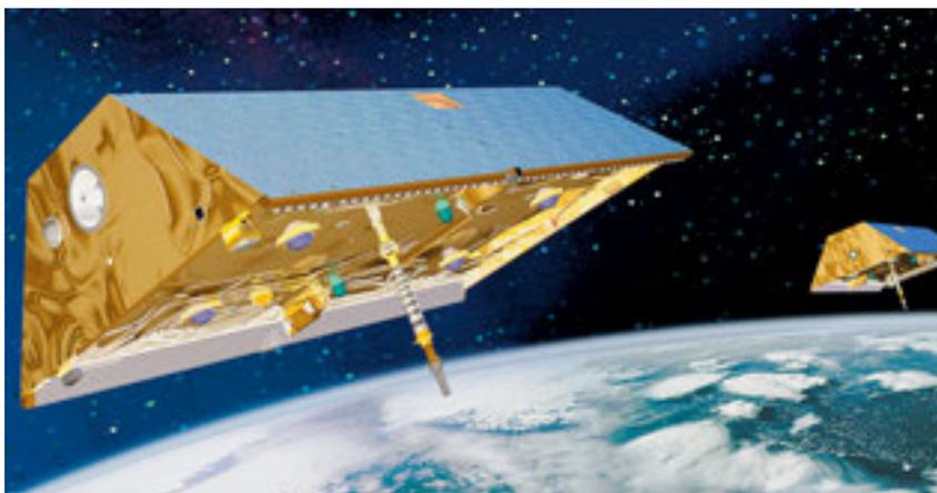
**Fig. 17: The twin Gravity Field and Climate (GRACE) Experiment** spacecraft shown in an artist's view. The two satellites circle the Earth on the same orbit some 220 km apart. A microwave ranging instrument monitors the distance between the two very precisely. It is the variation of this distance which yields an indication to the variability of the Earth's gravity field. (Credit: NASA).
