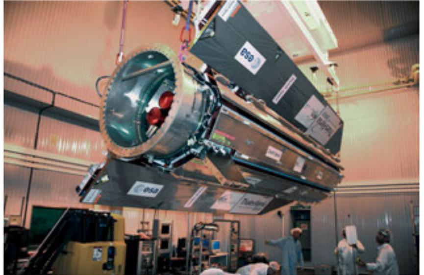
**Fig. 9: The GOCE spacecraft** undergoing final tests in the clean room at the Plesetsk Cosmodrome in Russia. (Credit: ESA).
